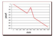
Figures 5. Roll Error in the Y axis with a lineal content and a "local pulse". The results went identical to the results that in theory should be obtained.
