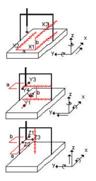
Figure 1. Positions of the ball beam to evaluate the yaw, pitch and position errors.
