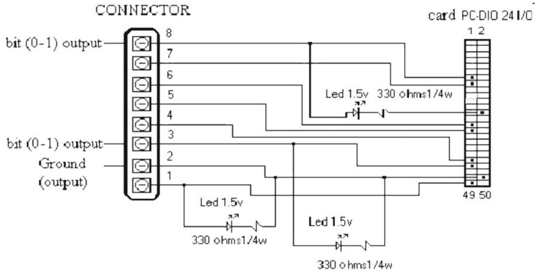
Figure 3. PC – control system interface card
