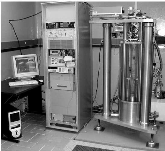
Figure 3. IMG/CENAM-HG6 mercury manobarometer photography.
