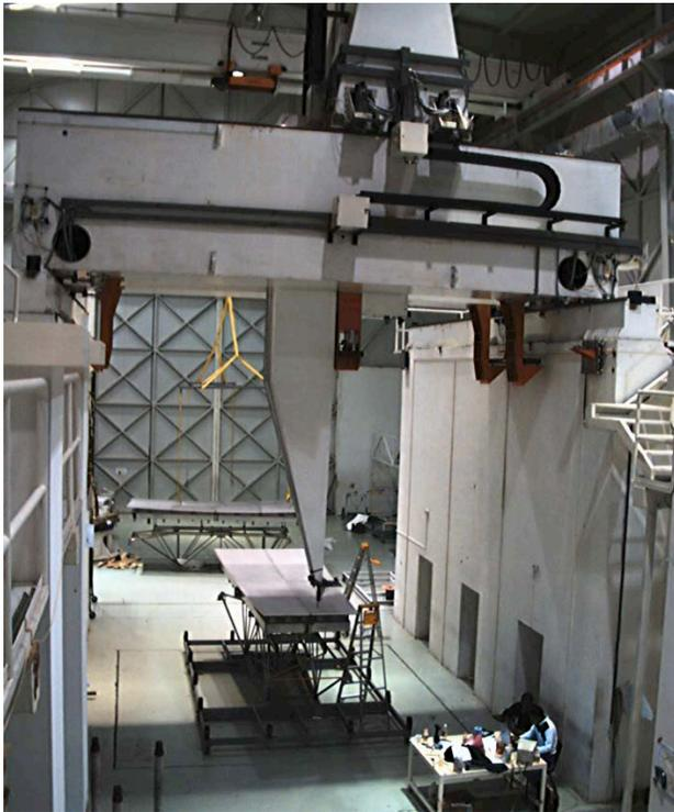
**Figure 1.** Measurement of an LMT primary reflector surface segment using the INAOE CMM.
