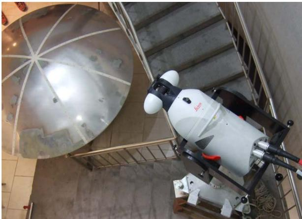
**Figure 6.** Secondary mirror with Leica tracker inside the antenna basement.
