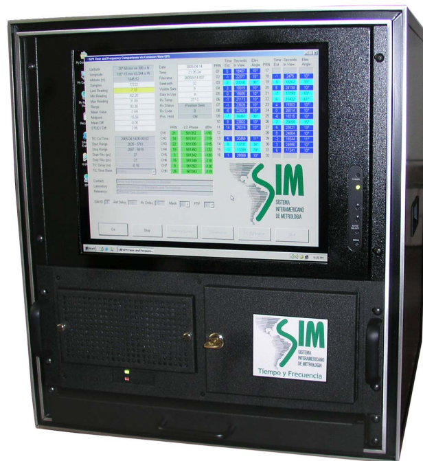
Figure 2. The SIM common-view GPS measurement system.
