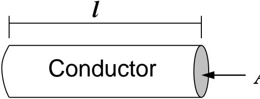
The diagram shows a cylindrical conductor with its length labeled as  $l$  and its cross-sectional area labeled as  $A$ .
