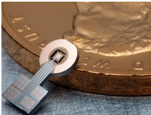
*Fig. 1. Photograph of PCR chip next to a USA penny for scale.*
