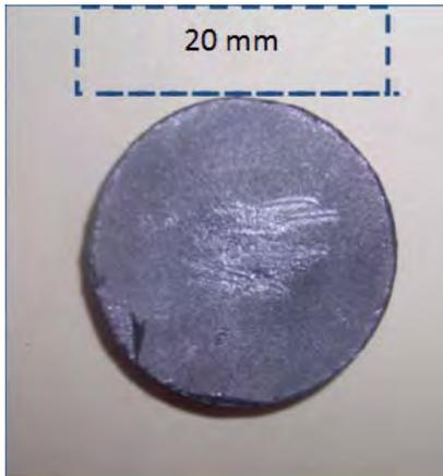
**Fig. 5** MCrAlY specimen like to a tablet.
