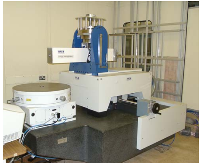
Fig. 4 The NPL/UCL swing arm profilometer.
