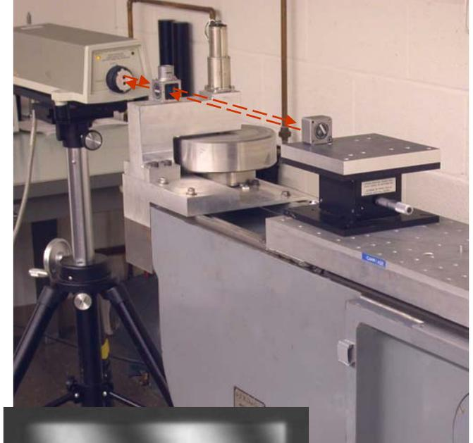
Fizeau interferometry: with less than 10 fringes across the field of view, accuracy of 1 part in  $10^4 = 0.3$  nm. (often employs unstabilized laser)
