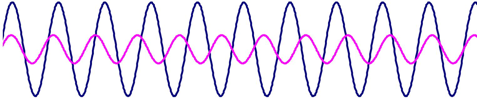
Small contamination (pink) at a different wavelength shifts phase of interference in a manner that varies periodically in space as the waves go in and out of phase.
