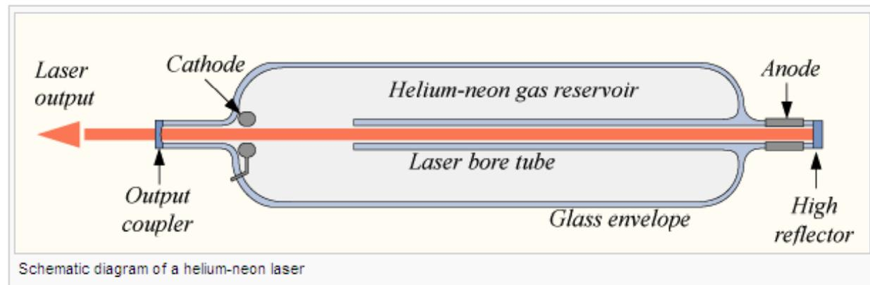
end of the glass tube. A current of 5 to 100 mA is typical for **CW** operation.<sup>[3]</sup> The **optical cavity** of the laser typically consists of a plane, high-reflecting **mirror** at one end of the laser tube, and a concave **output coupler** mirror of approximately 1% transmission at the other end.
