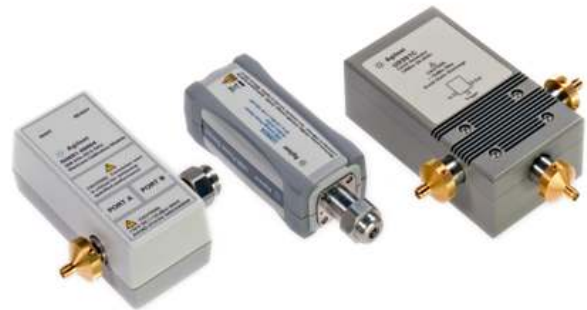
Figure 4: Calibration standards used for calibrating a NVNA, showing (left to right) a vector calibration standard (ECal module), USB power sensor, and phase reference which are used to analytically remove the systematic errors from the measurements.
