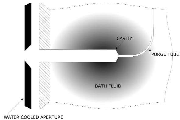
**Fig. 1** Diagram of Hart's Liquid Bath Blackbodies.
