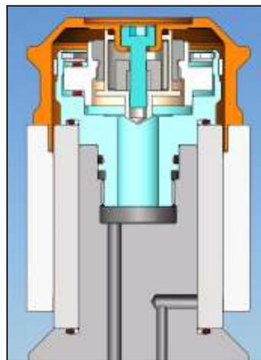
**Figure 3** Drawing of piston-cylinder assembly and mounting post
