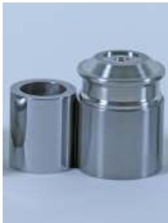
**Figure 2** Picture of the 20 cm<sup>2</sup> area piston-cylinder
