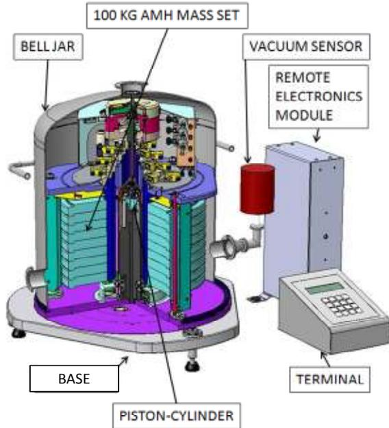
**Figure 1** PG9607 Platform Main Components
