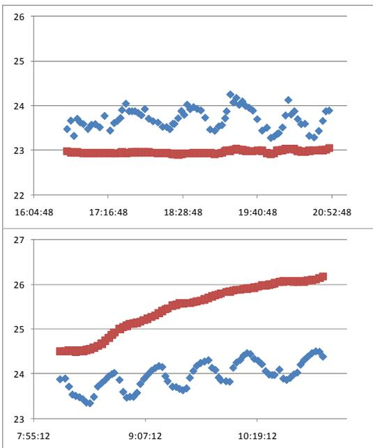
**Figure 6.** Piston-cylinder temperature (red) and ambient temperature (blue) of a PG9607 (top) and a PG7601 (bottom) performing the same pressure test.
