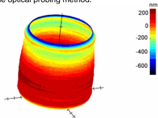
**Fig. 2** Helical scan of the full surface of a pressure gauge piston performed with the optical probe system.
