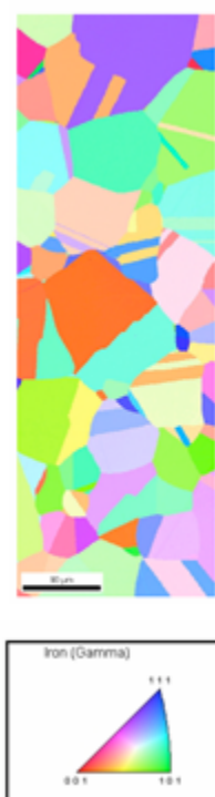
Fig. 3. EBSD orientation map (scale 90 μm) for the austenitic sample and inverse pole figure.
