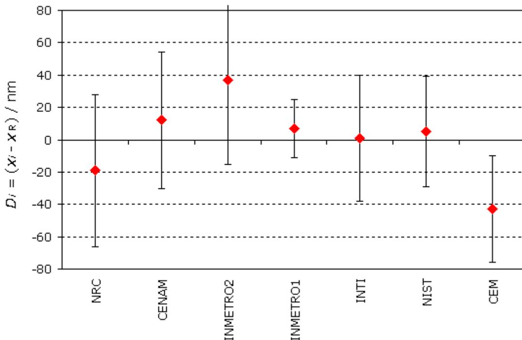
**MEASURAND : Central length of short gauge block measured by interferometry according to ISO 3650; gauge block material: tungsten carbide**
