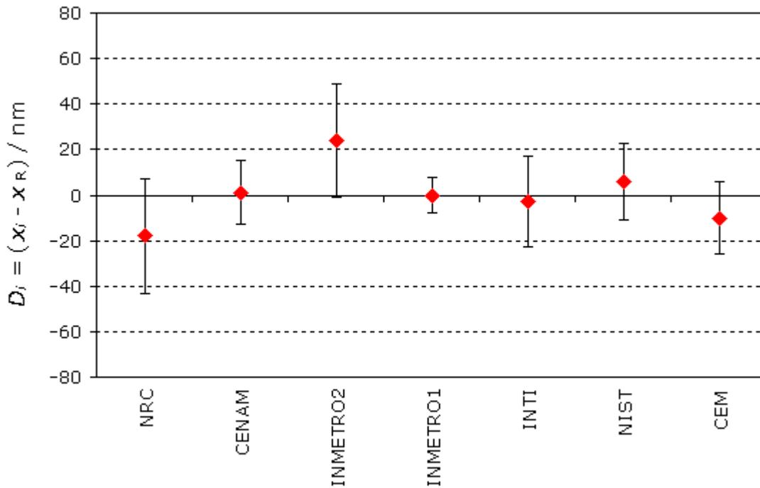
**MEASURAND : Central length of short gauge block measured by interferometry according to ISO 3650; gauge bolck material: steel**
