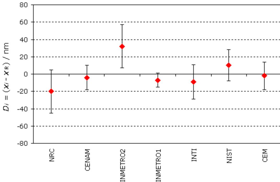
**MEASURAND : Central length of short gauge block measured by interferometry according to ISO 3650; gauge block material: steel**
