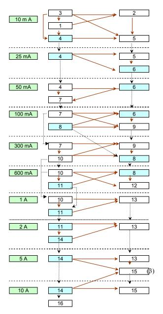
Fig 1 - Overdetermined AC-DC current step-up. In light blue is also shown one possible direct scheme with only one TC jumping between levels.
