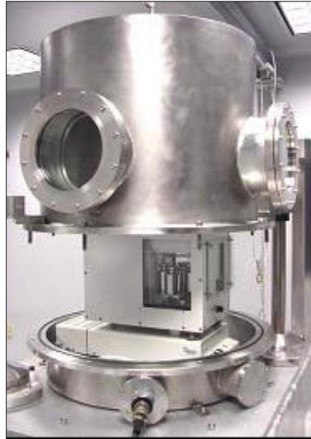
Figure 1. Sealed chamber of the CENAM mass laboratory. The chamber is open to show a balance inside.
