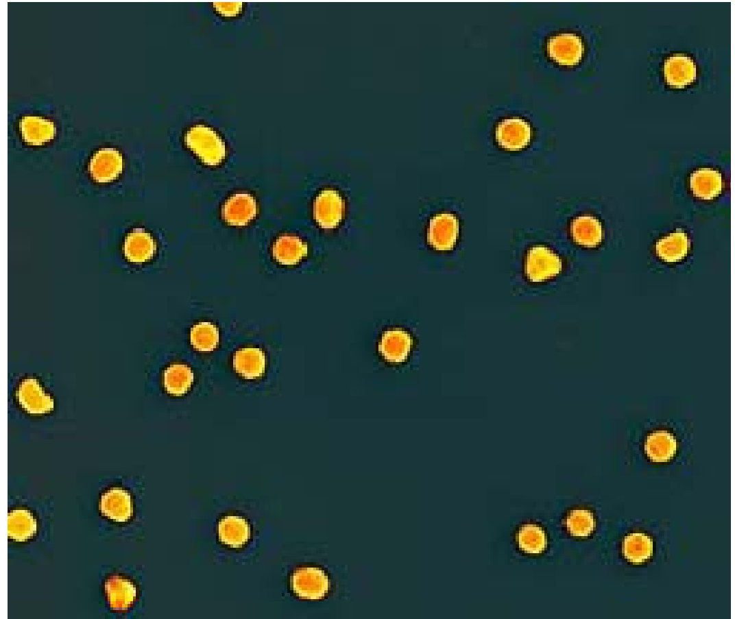
A. Vladar, SEM of RM 8012 particles
