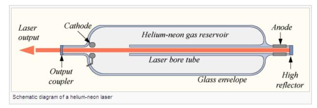
end of the glass tube. A current of 5 to 100 mA is typical for CW operation.<sup>[3]</sup>. The optical cavity of the laser typically consists of a plane, high-reflecting mirror at one end of the laser tube, and a concave output coupler mirror of approximately 1% transmission at the other end.
