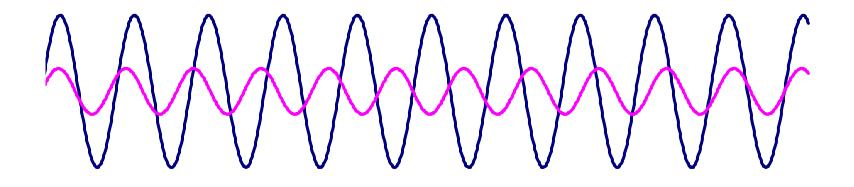
Small contamination (pink) at a different wavelength shifts phase of interference in a manner that varies periodically in space as the waves go in and out of phase.
