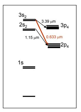
Red transition of the common He-Ne laser: fixed by atomic properties of the neon atom
