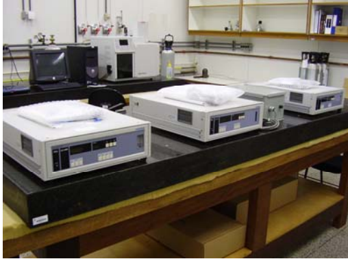
Fig. 3. Non-dispersive infrared and quimi-luminescent analyzers.
