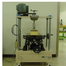
Torque calibration machine (0.1 %)
