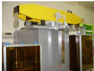
Torque standards in KRISS (0.005 %)
