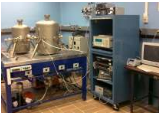
Figure 2. Static expansion system at CENAM.
