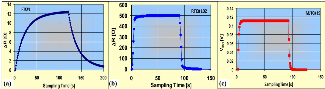
**Figure 8.** (a) Time constant of an RTC implemented on a rather thick wafer. (b) An RTC' time constant micro-machined from a 20µm thick active layer. (c) Typical time constant of the PMJTCs by the PTB-Germany.
