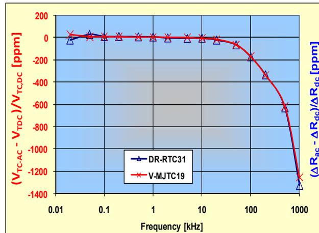
**Figure 9.** AC-DC conversion difference recorded for the HP-calibrator versus frequency. The MJTC's thermopile voltage difference (red) and the RTC's change in resistance of the detecting silicon resistor (blue).
