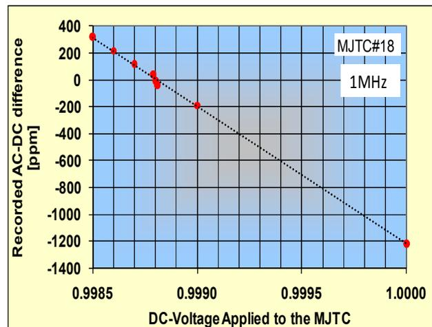
Figure 7. Recorded AC-DC differences versus the DC-voltage applied to the MJTC#18, at 1MHz. Nominal AC-voltages of 1V result in a negative difference indicating that these AC-signals produce less heating (a lower output voltage across the thermopile) than that produced by the 1V DC-signal. If the DC-voltage is lowered to approximately 0.9988V, the AC-DC difference becomes near-zero, becoming positive for lower DC-voltages.
