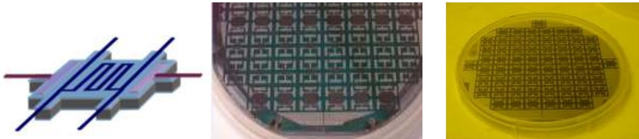
**Figure 3.** Basic structure of the RTC concept, as designed and fabricated. The heater (Cu-Ni) lays on top of the detector element (Si-resistor)
