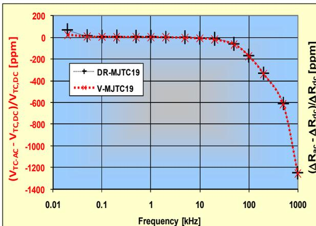
**Figure 10.** AC-DC conversion difference recorded for the HP-calibrator versus frequency, established from the output voltage (red) and the resistance (black) of the MJTC’s thermopile.
