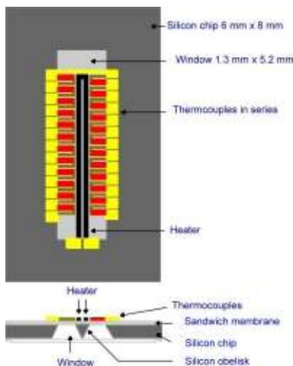
**Figure 1.** Configuration of PTB's Planar-MJTC, where 100 thermocouples in series (thermopile) surround the bifilar element or heater (center). Top and side view. <http://www.ptb.de/en/org/2/21/212/pmjtc.htm>
