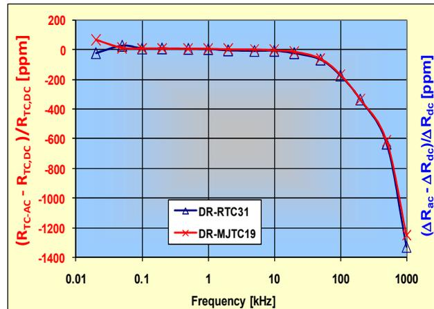
**Figure 11.** AC-DC conversion difference recorded for HP-calibrator versus frequency, established from the resistance of the MJTC’s thermopile (red) and the resistance of the RTC (blue).
