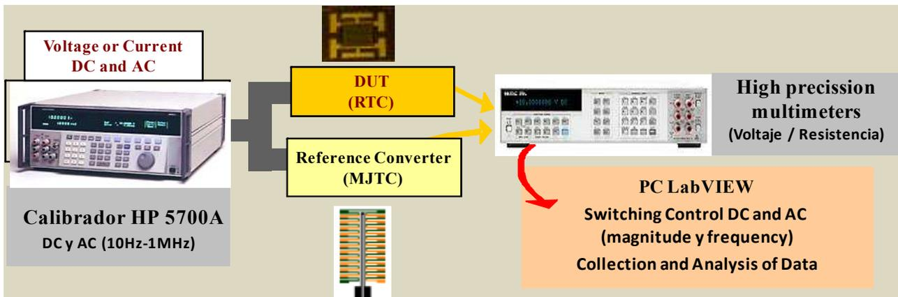
**Figure 5.** Schematic of the test circuit used for the characterization of the AC-DC transfer difference of the RTC.
