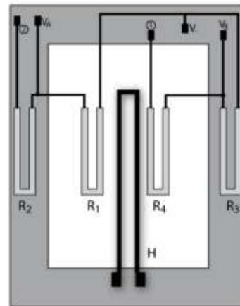
**Figure 2.** Configuration of a resistive type thermoconverter[6] using two  $\text{VO}_2$ -resistors on the sides of the bifilar NiCr-heater, and configured within a Wheatstone bridge.
