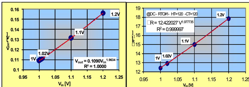
**Figure 4.** Determination of the transfer constant,  $n$ , for both the MJTC (left) and the RTC (right). The value obtained for  $n$  of the MJTC concurs with the value reported by the manufacturing Lab. Both show an  $n$ -value very close to 2, with good correlation coefficient of the power curve fit.
